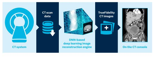
Figure 8: Reconstruction flow of deep learning image reconstruction.
