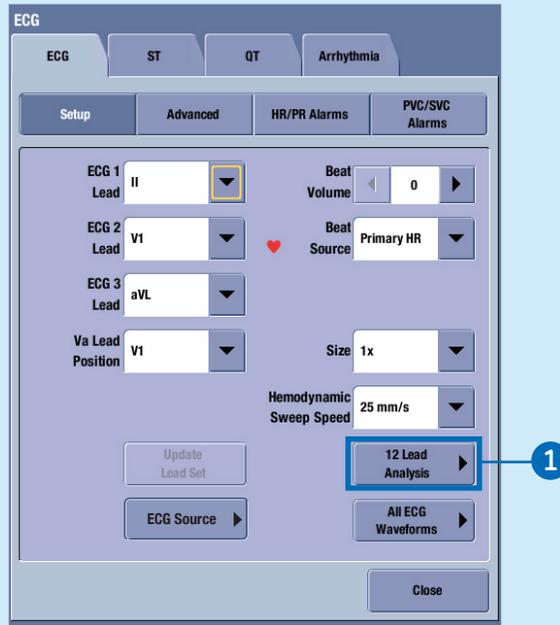
Figure 12 Accessing 12 Lead Analysis
