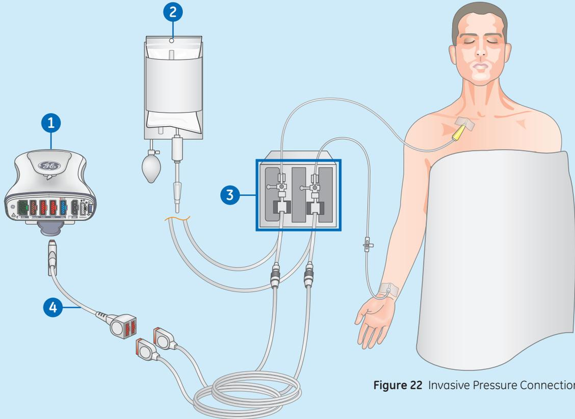
Figure 22 Invasive Pressure Connections
