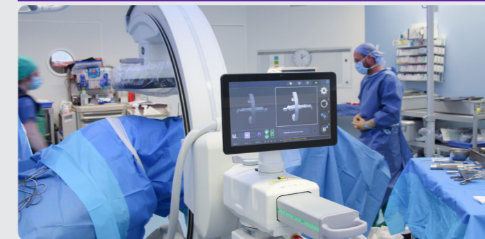
Set up of patient orientation, imaging acquisition mode, dose level and 3D volumetric images reconstruction option. Activation of the connectivity with the integrated Brainlab navigation system.
