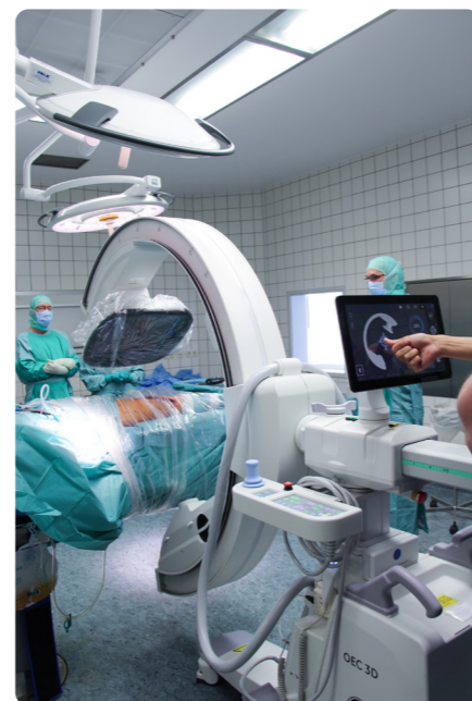
Starting 3D collision check on OEC 3D.
