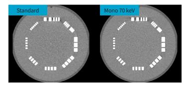
Figure 5: Comparison of TrueFidelity DL images for single-energy (left - 120 kV) and dual-energy (right - GSI, monochromatic 70 keV) on the section of the Catphan phantom with visual resolution bars. Images are with the Standard kernel with 0.625 mm slice thickness and the DL-H setting, illustrating similar visual resolution, noise, and texture, without aliasing or artifacts.
