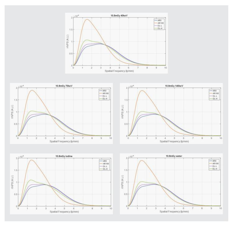
Figure 10a: Normalized Noise Power Spectrum performance across GSI image types at fixed dose (10.8 mGy) comparing TrueFidelity DL for Spectral imaging at the Low and High settings (DL-L and DL-H), ASIR-V 100% (AR100), and FBP (AR0). Graphs show 40, 70, 140 keV (top), as well as iodine (water) and water (iodine) basis materials (bottom). Measured from 20 cm centered | Water phantom.
