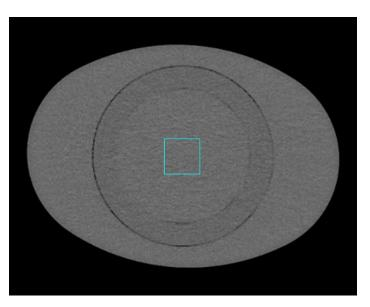
Figure 3: Uniformity section of the Catphan 600 with an added annulus to simulate the attenuation of a typical adult body, with a 4x4 cm centered ROI for noise measurements.
