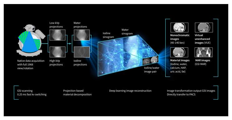
Figure 2: GE leverages deep learning reconstruction engine to generate GSI images.
