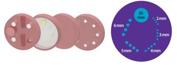
Figure 6a: 3D rendering of the modules of the ACR CT accreditation phantom (Gammex 464) and schematic of the low contrast section for CNR measurements.
