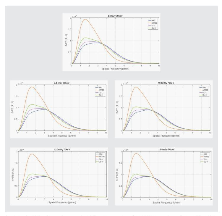
Figure 10b: Normalized Noise Power Spectrum performance across dose levels from 15.6 down to 5.1 mGy comparing TrueFidelity DL for Spectral imaging at the Low and High settings (DL-L and DL-H), ASIR-V 100% (AR100), and FBP (AR0). Measured from 20 cm centered | Water phantom.
