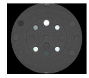
Figure 7: Gammex Multi-Energy CT phantom (left) used to assess MD quantitative accuracy, showing the water, iodine, and cortical bone inserts with their respective measurement ROIs in the iodine (water) image (right).
