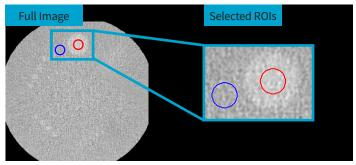
Figure 6b: Illustration of ROI placement for CNR assessment, ROI, in red and ROI, is in blue.
