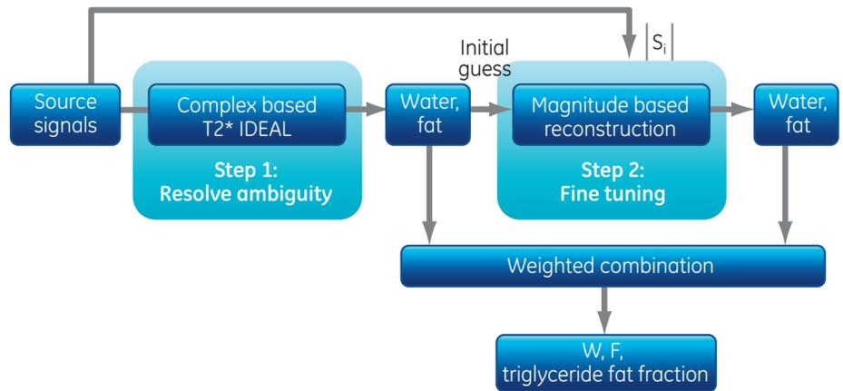
**Figure 6.** Flow diagram of the complex-based and magnitude-based hybrid approach. The second step relies on the results from the first step for initial conditioning of the fit. The results from the two steps are combined to provide robust and accurate water-fat separation.
